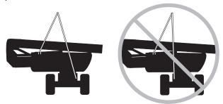
Attach the rigging to the 2 chassis lifting points farthest from the turntable lifting point.
